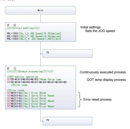
(2) No.1 Motion control: Motion Control Normal Task [Automatic Start]
