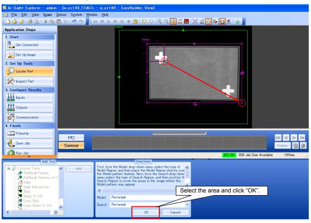
3) Set the offset values so that the image processing result (X- and Y- coordinates) for the regular position becomes "0.0".
