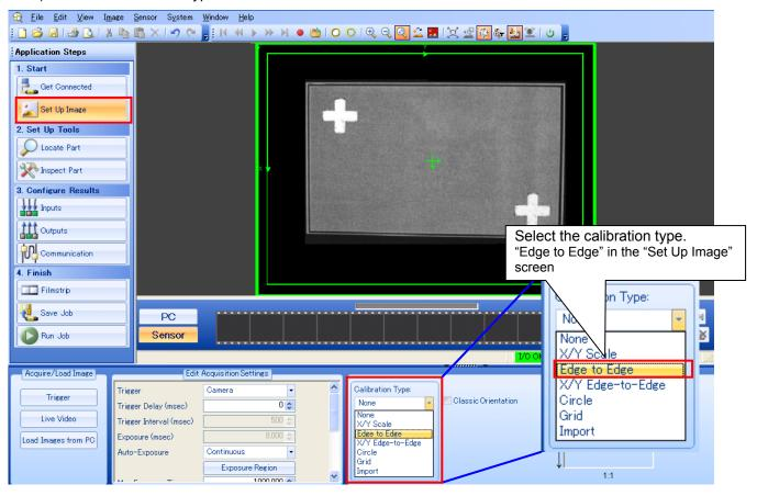
2) Define the actual dimensions of the work piece by its edges.
