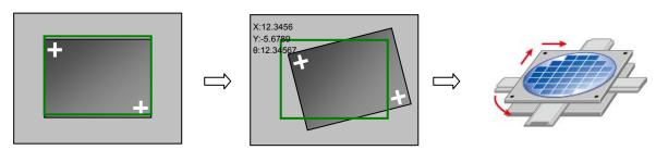
The In-Sight® Explorer vision tool Is used to register the image of the normal position of the work piece as a pattern.
