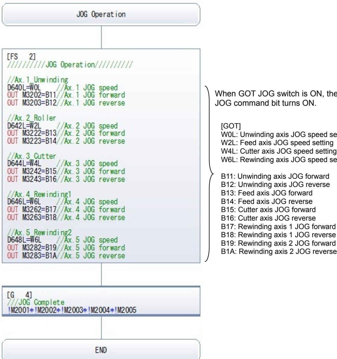
When GOT JOG switch is ON, the corresponding JOG command bit turns ON.
