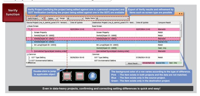
The project Verify function allows for detailed verification by object, not only by projects/screens. Users can also confirm results in the Verify Result window and jump to the applicable object on the screen. In the Verify Result window, as you can export Verify results and narrow down by screen type, even in data-heavy projects confirming and correcting setting differences is quick and easy.
