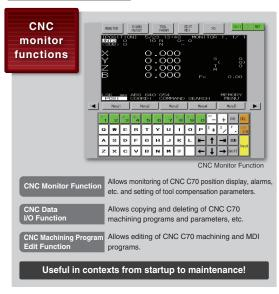
CNC monitor functions can be used with the GOT2000 Series.
