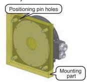
Table type (with positioning pin holes)
