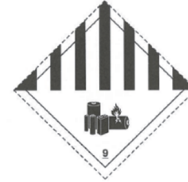
Figure 2. Lithium battery hazard label example
