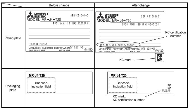
Figure 1. Addition of indications to the rating plate and packaging plate
