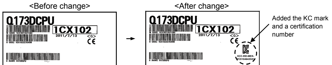
Figure 2. Example of KC mark and certification number indicated on the packing box
