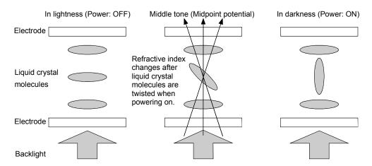
The TN LCD expresses gradation using the twist orientations of liquid crystal molecules as described above; however, color reversal occurs depending on a viewing angle.
