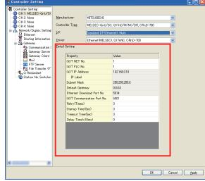
By changing the Ethernet interface from the extension interface to the standard interface, the configuration of the extension units may require changes. Therefore, change the controller setting overall.
