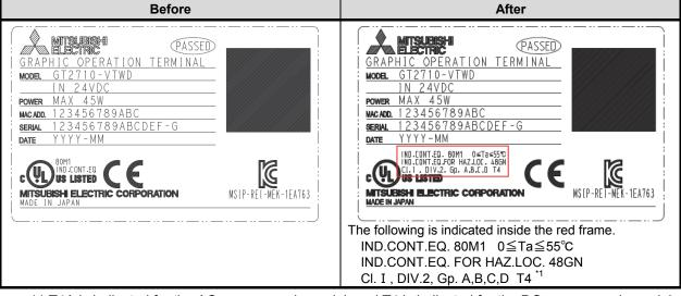
\*1 T4A is indicated for the AC power supply model, and T4 is indicated for the DC power supply model.
