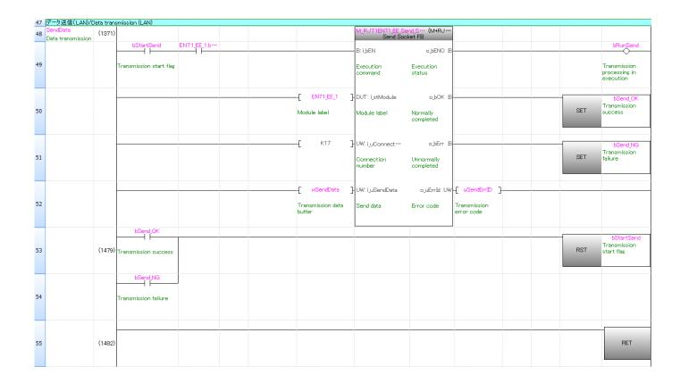
For the operation of M+RJ71EN71\_EE\_Send\_Socket FB, refer to "MELSEC iQ-R Ethernet, CC-Link IE, and MELSECNET/H Function Block Reference" for the Mitsubishi Electric programmable controller. In addition, the above program is quoted from "7.1 Communication Examples of Ethernet" of "MELSEC iQ-R Ethernet/CC-Link IE User's Manual (Startup)" for the Mitsubishi Electric programmable controller. For details, refer to that manual.
