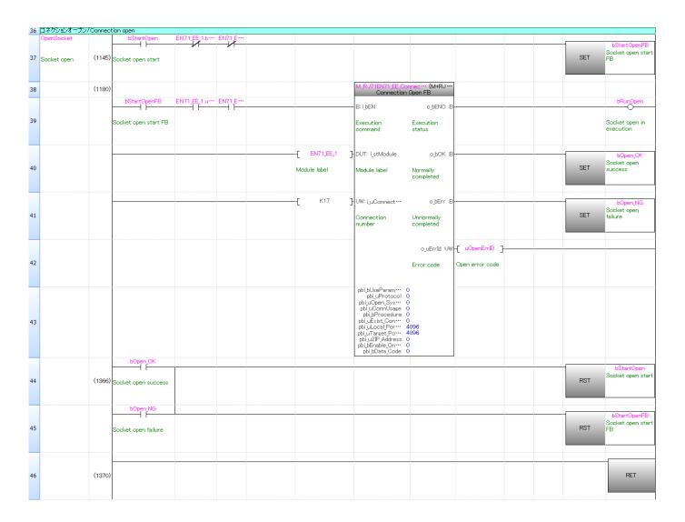
For the operation of M+RJ71EN71\_EE\_ConnectionOpen FB, refer to "MELSEC iQ-R Ethernet, CC-Link IE, and MELSECNET/H Function Block Reference" for the Mitsubishi Electric programmable controller. In addition, the above program is quoted from "7.1 Communication Examples of Ethernet" of "MELSEC iQ-R Ethernet/CC-Link IE User's Manual (Startup)" for the Mitsubishi Electric programmable controller. For details, refer to that manual.
