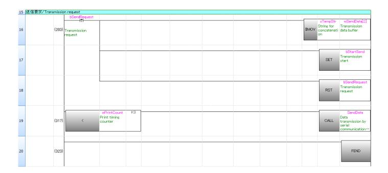
Row number 16: Sub-routine Copy transmitted data prepared at SetTransData to the transmission data array "wSendData".
