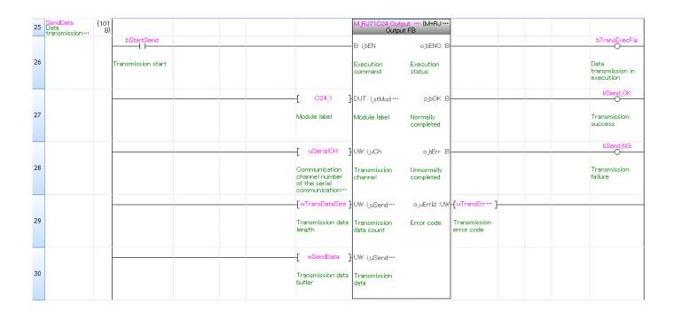
The data is transmitted with the number of bytes which is shown in the transmit data length wTransDataSize stored in wSendData [].
