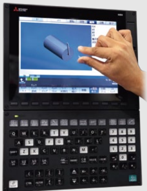
The display unit incorporates touch panel operation whereby the user merely swipes his/her finger across the screen, just like a smartphone, in order to zoom in/out and move the cursor, thus speeding up the process dramatically.
