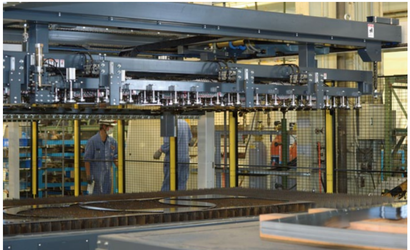
After cutting, parts are placed on a pallet by over 200 suction pads, and the scrap is carried back to stock shelves using a special-purpose forklift.
