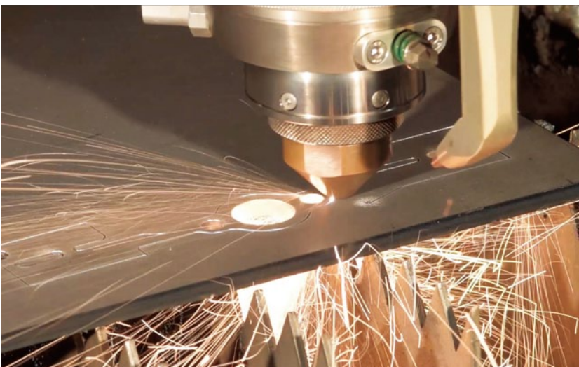
Processing using the eX-F60.
