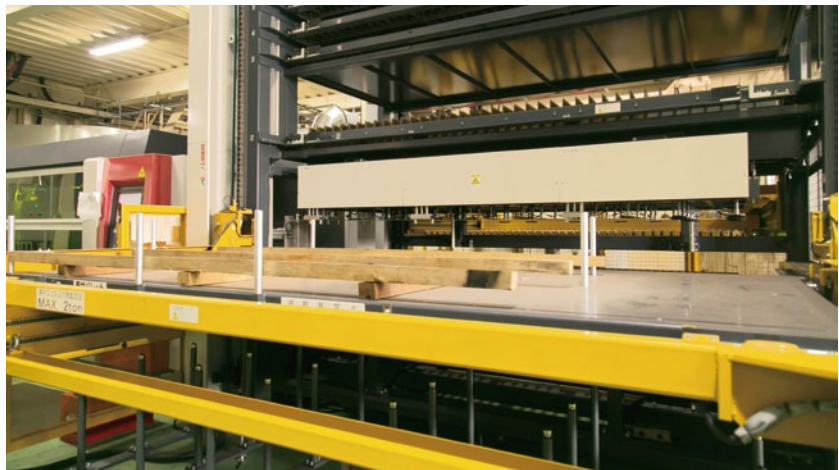
When Ueno Tekko installed the eX-F60, it also installed the 30SCX-eX-F, a stocker capable of high-speed sheet changing. This significantly improved work efficiency as material can be automatically loaded into the machine.
