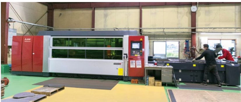
ML3015eX-F40 2D fiber laser processing machine by Mitsubishi Electric purchased by Nittetsu in July 2016. 4kW power
