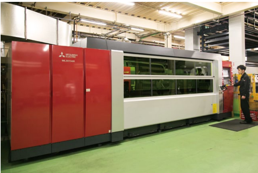
The Mitsubishi Electric eX-F60 2D laser processing machine installed at the end of 2015. With an output of 6kW, it can cut brass, copper and aluminum, which had been difficult using CO 2 .
