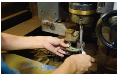
The wire-cut EDM robot system jointly developed with Mitsubishi Electric in 2013 to manufacture atypical electrodes. Playing an effective role in high-accuracy die manufacturing.
