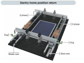
After the master and slave axes pass their respective dogs, the gantry home position return stops both of the axes at the Z-phase of the master axis.
