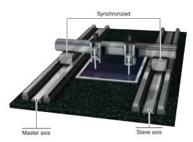
Motion Control Software enables tandem operation where the same commands can be outputted to master and slave axes.
