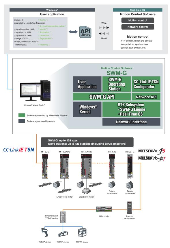
\* Motion Control Software can function as a master station of CC-Link IE TSN.
