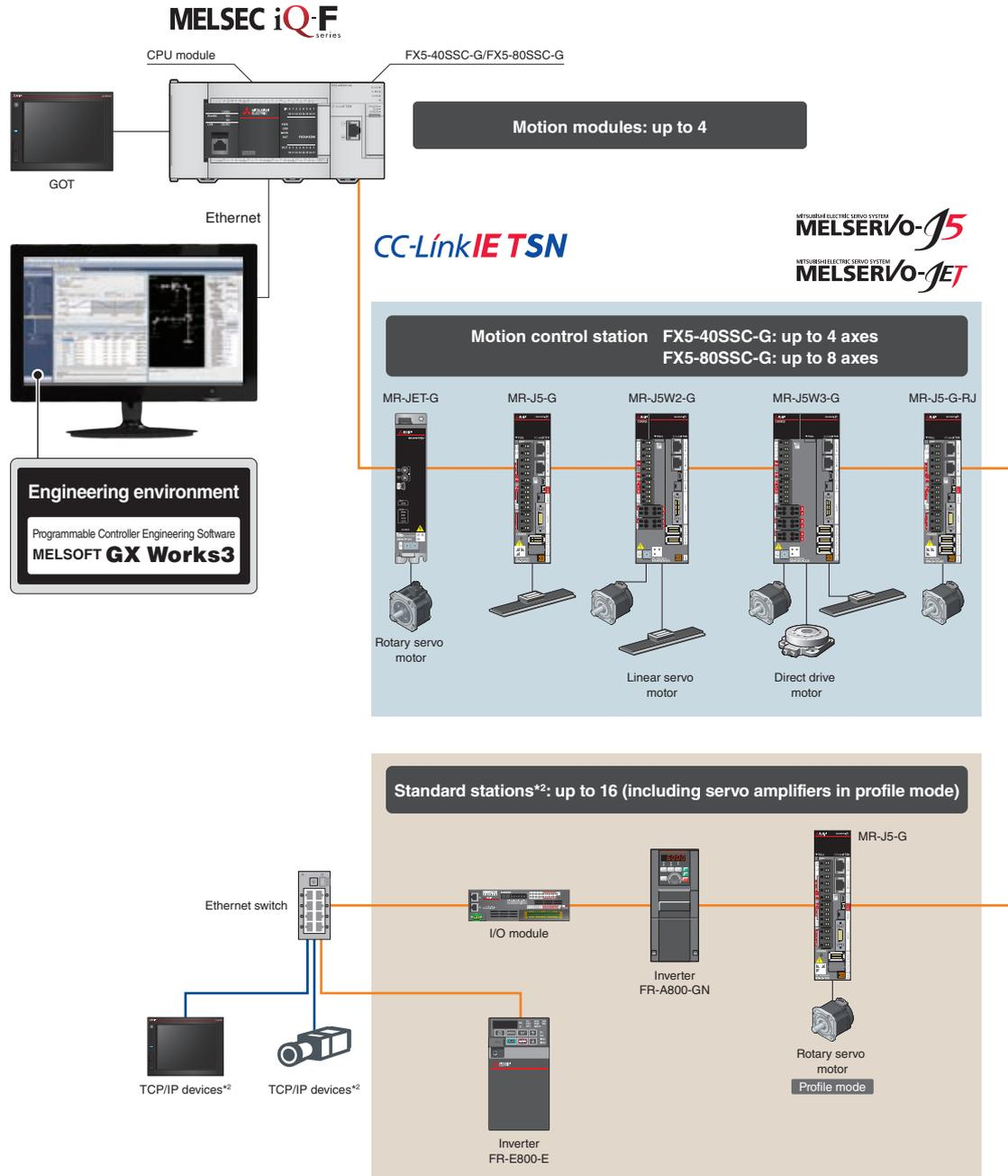
\*1. The Motion modules are not provided with the following functions: sub-master station, local station, multi-master configuration, and backup/restore function.
