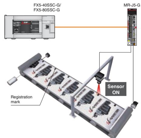
This function latches data responding to a trigger signal input to a servo amplifier. The compensation amount is calculated based on the latched data, and the error is compensated using a compensation axis.
