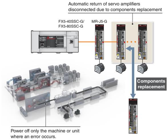
When slave stations are back to normal status after disconnected due to a data link error, this function automatically returns the disconnected stations to the network and restarts data link. When defective components need to be replaced in one of the machines in a production line or one of the units in a machine, only the machine or the unit can be partly turned off without powering off the whole system.
