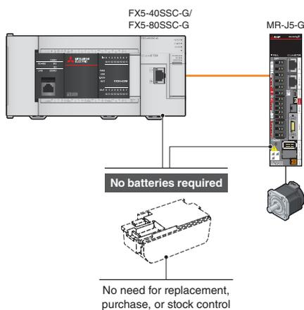
The Motion module and the servo amplifier can be operated without a battery.\*1 Maintenance costs are reduced as a result of eliminating the battery replacement and stock control.
