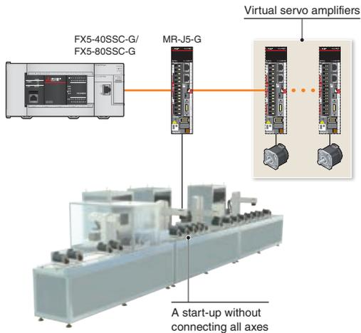
The virtual servo amplifier function enables operations of a virtual servo amplifier as if an actual unit is connected. When the virtual servo amplifier is set as a servo input axis of synchronous control, the Motion module executes synchronous control with virtually generated input commands. In addition, this function is used to simulate an axis without an actual connection.
