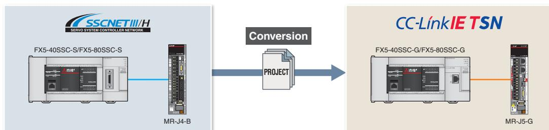
\* Parameter settings for the network and servo amplifiers are required.
