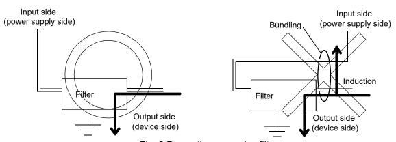
Fig. 2 Precautions on noise filter
