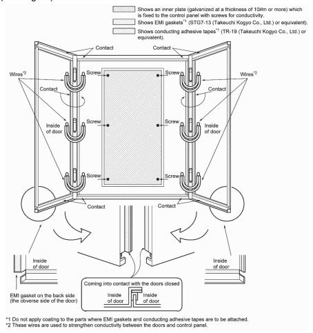
Fig. 1 Example of Control Panel Inside
