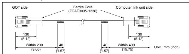
• The cable length must be within 15m.
