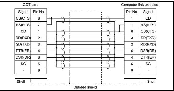
• When D-sub 25-pin is used for the connector of the computer link unit. (AJ71QC24(-R2), AJ71UC24)
