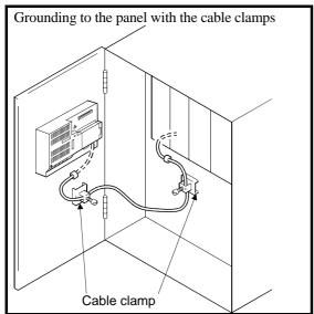
For RS-232C cable, ground the braided shield onto the panel with the cable clamp (AD75CK).
