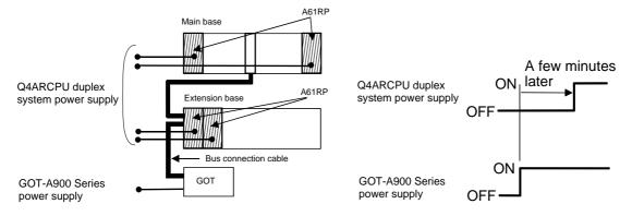
It is recommended to build an external circuit in advance.
