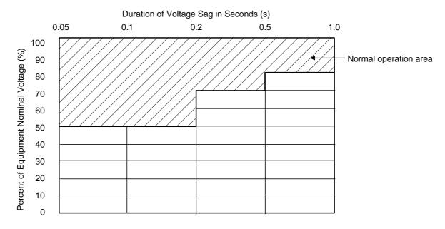
SEMI-F47 defines that the equipment must continue to operate (voltage sag ride-through capability) without interrupt during voltage sags above the line (upward diagonal line area).
