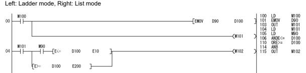
In the ladder block starting from step 104, the ANDE<= instruction of step 106 and the ORE>= instruction of step 110 are not executed when M101 (valid data flag) is off.
