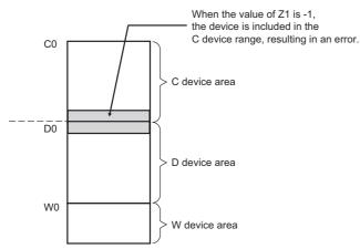
When an error is detected, check the index modification value (value of Z1 in the above example) and remove the error cause.
