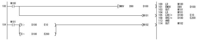
In the ladder block starting from step 104, the floating-point data comparison instructions of steps 105 and 109 are not executed when M101 (valid data flag) is off.
