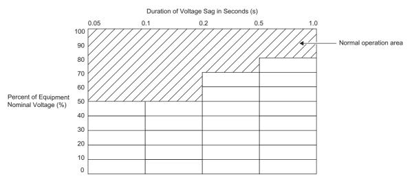
SEMI-F47 defines that equipment must be able to continue to operate without interruption during voltage sags shown in the above shaded area (voltage sag immunity).
