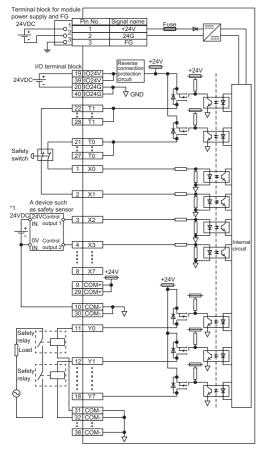
\*1 The power supply of 24VDC can be applied from the COM+ terminal.
