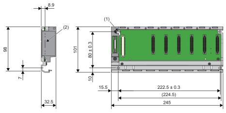
(1) Four mounting screws (M4×14)(2) Module face to be mounted
