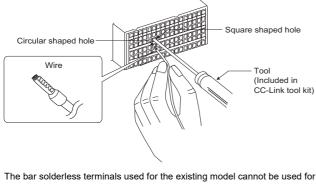
The bar solderless terminals used for the existing model cannot be used for the CC-Link IE TSN remote I/O module with safety functions of the alternative model.
