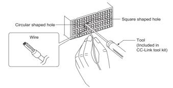
The bar solderless terminals used for the existing model cannot be used for the CC-Link IE TSN remote I/O module with safety functions of the alternative model.
