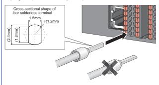
Use the recommended bar solderless terminals depending on the wire diameter.
