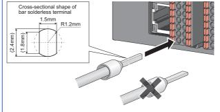
Use the recommended bar solderless terminals depending on the wire diameter.
