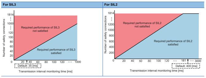
Examples of settings on a system configured using the MELSEC iQ-R series Safety CPU and the safety function module for the master station and the CC-Link IE Field Network remote I/O module (with safety functions) for the remote device stations
