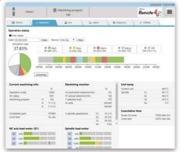
The utilization rate and operation data of each machine are displayed. Visualization and analysis helps you improve production process.
