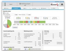
The utilization rate and operation data of each machine The selected machine's load, power consumption and are displayed. spindle unit temperature are displayed in graphs. Visualization and analysis helps the end user improve The end user can use the data in analysis to improve machining quality and reduce running costs.
