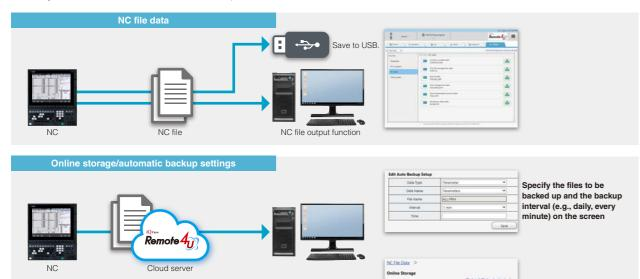
Files are automatically backed up to the cloud based on predefined conditions (Max, 100 MB, Old files are deleted from the oldest.)
