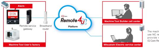
The machine tool users can also use NC remote service when you provide remote service using iQ Care Remote4U.
