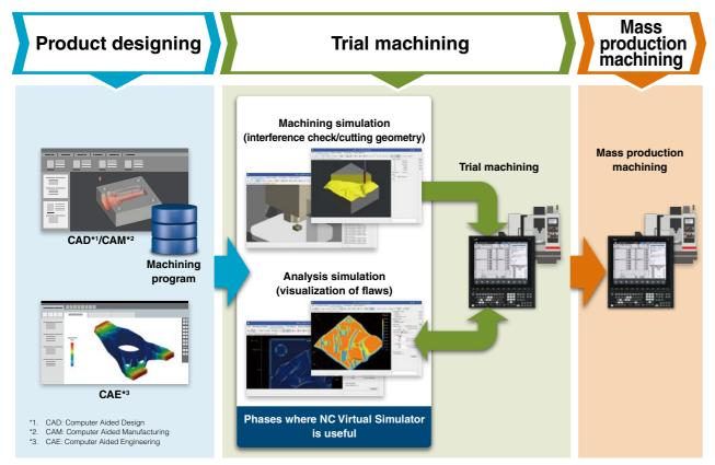
Diverse features allow you to validate machining programs, verify work instruction data, and analyze the flaws in the surface finish to help you identify and correct issues at trial machining stage.
