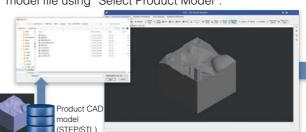
Simulation result is superimposed with the product CAD model.
