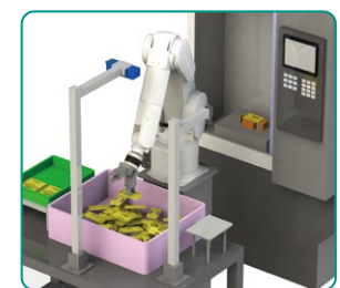
Picking from a large pallet (Fixed camera)
