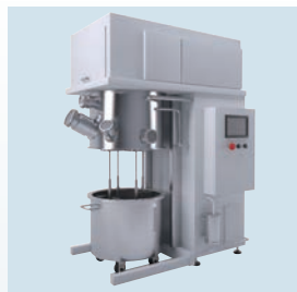
Stirring (lithium-ion battery production line)
