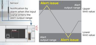
By using the input signal error detection function and alert output function (process alarm/rate alarm), the operator can easily monitor the status of connected equipment.
