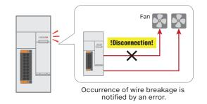
Disconnection detection function is enabled only when the analog output range is 4 to 20 mA, 0 to 20 mA or the user range (current).
