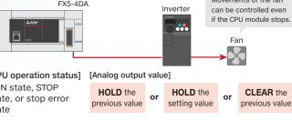
Sets whether to clear the current analog output value, or hold the previous value or the setting value when the CPU module operating status is Run, Stop, or Stop Error.
