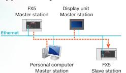
Each master station can access the FX5 module (having the slave function).
