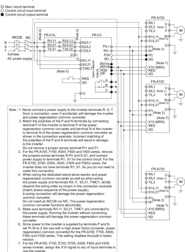
8. You can connect up to six inverters to one power regeneration
