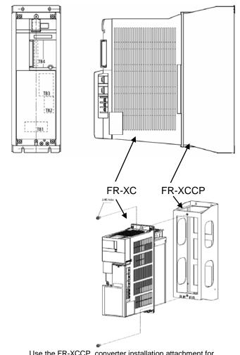
Use the FR-XCCP, converter installation attachment for enclosure (option), to install the multifunction regeneration converter inside an enclosure.
