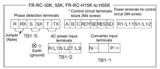
(Note) Do not remove the jumpers except when taking measures for preventing overcurrent due to power supply distortion.
