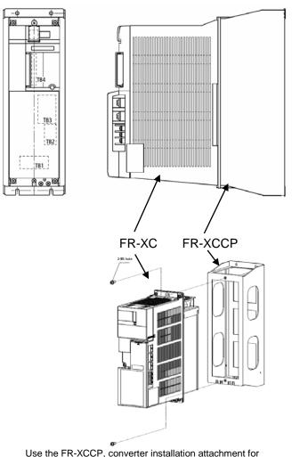
Use the FR-XCCP, converter installation attachment for enclosure (option), to install the multifunction regeneration converter inside an enclosure.
