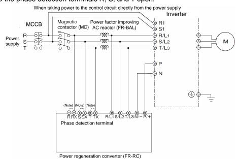
Note: When not using the phase detection terminals, do not remove the jumpers across R and RX, across terminals S and SX, and across terminals T and TX.
