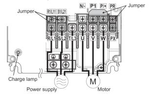
M5 (M4 for terminals PR, PX, R1/L11, and S1/L21)
