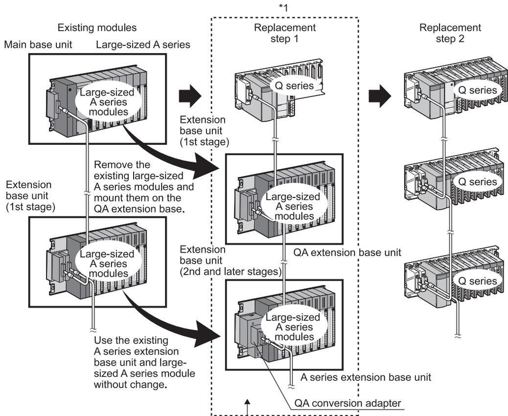
The existing A/QnA series modules can be used by mounting them on the QA(1S) extension base module.
