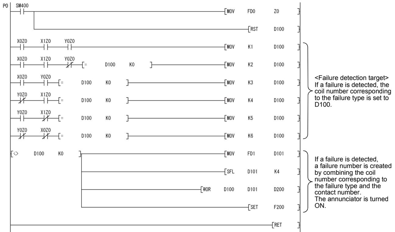
**(4) Replacement method when failure detection ladder patterns are changed by the CHK CIR and CHK END instructions**
