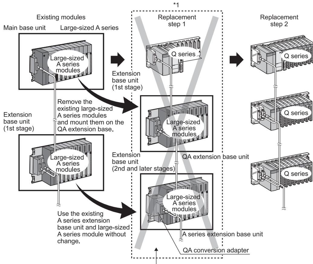
The existing A/QnA series modules cannot be used by mounting them on the QA(1S) extension base module.
