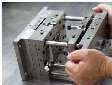
A completed die for producing moldings used in precision electronic components.
