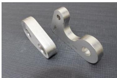
An example of stainless steel processing. The part on the left is 20mm thick and the part on the right is 16mm thick. Seiryoh guarantees being able to bore holes the same size as material thickness and can reduce the hole diameter by half depending on the application.
