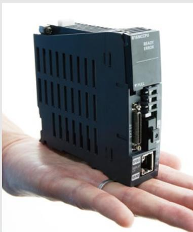
The size of the main unit is a mere 110 × 106 × 27.8mm. Various functions that have been significantly enhanced are provided in a compact body.
