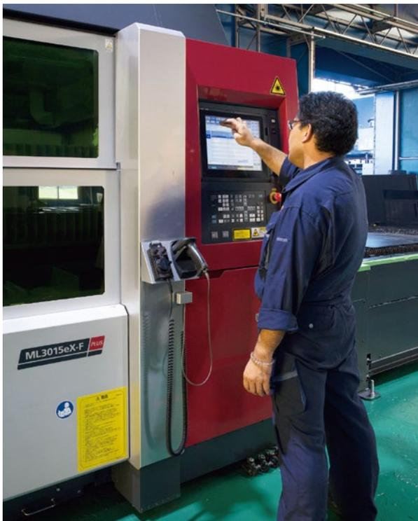
"ML3015eX-F60" - The fiber laser machine with an output of 6kW introduced in March 2017. This machine is preferred for two-dimensional machining.
