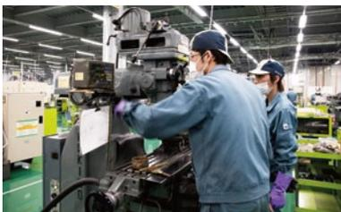
Skills are essentially passed on through OTJ. The photo shows a cemented carbide tool being machined by a worker during OTJ.
