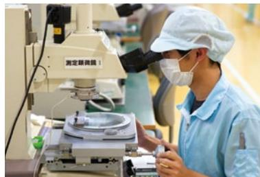
The die inspection process. Completed dies have a high machining accuracy of within  $\pm 1 \mu\text{m}$ .
