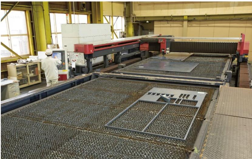
The large ML6030XL-45CF-R laser processing machine is capable of processing materials up to a size of 6,100mm x 3,050mm. It also comes with a pallet changer.
