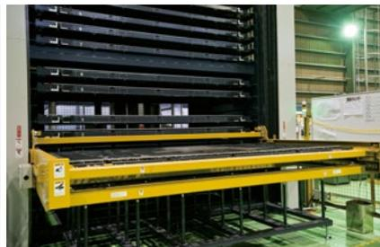
ML3015eX-F60 6kW fiber laser processing machine processing a workpiece (left). In the center is a part manufactured by processing steel plate. Of the two laser processing machines introduced, one has a 15-step pallet changer capable of automatically loading/unloading steel plates into the machine (right).
