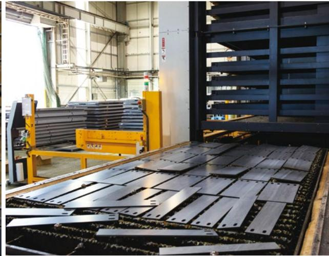
The fiber laser processing machines are equipped with a 15-step pallet changer. This makes efficient around-the-clock operation possible.
