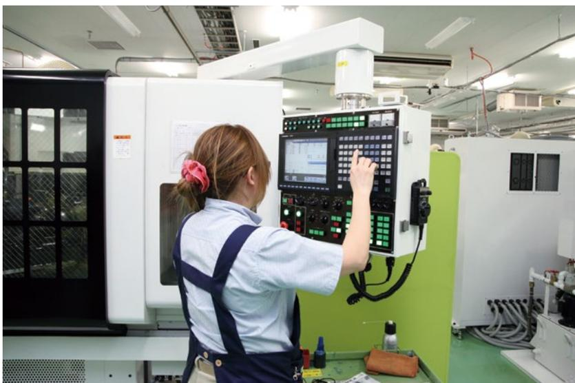
TGM – a tool grinder developed by NS TOOL in-house. It utilizes the Mitsubishi Electric M750VW as its CNC.
