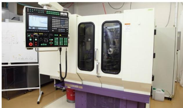
The first TGM unit completed in 2006. It is currently installed in NS TOOL’s development center and is used for prototyping new cemented carbide end mills products.
