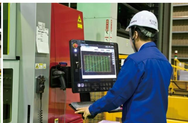
ML3015eX-F60 – Mitsubishi Electric 6kW fiber laser processing machine introduced in 2018. Equipped with both a 15-step pallet changer and 6-step sheet changer, this machine is capable of automatic operation, even at night.
