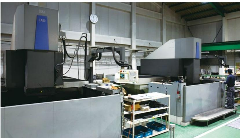
In line with the company's policy, "Always introducing two processing machines at a time," Houden Engineering also installed two large EA50 die-sinking EDMs.
